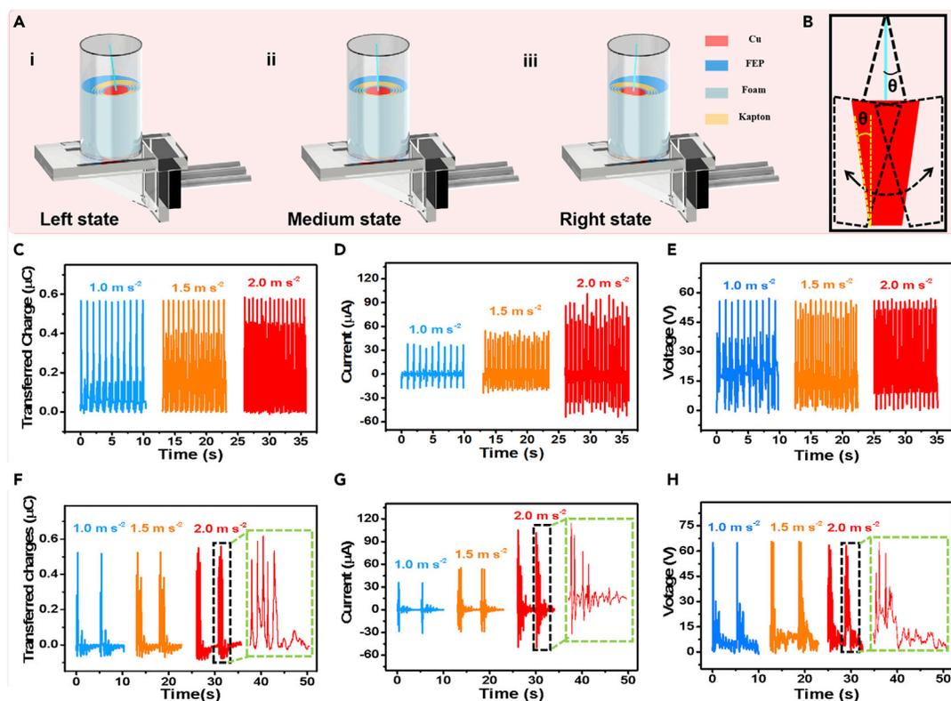
**Figure 2. Output performance of AR-TENG system driven by linear motor**
