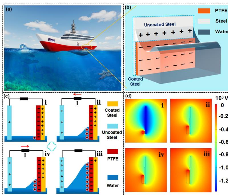
**Figure 1.** Structural design and working mechanism of the SL-TENG. (a) Device configuration of the SL-TENG installed on the hull. (b) Schematic representation structure for the SL-TENG. (c) Electricity generation principle of the SL-TENG. (d) Voltage potential distribution of the SL-TENG at different states by COMSOL simulation.
