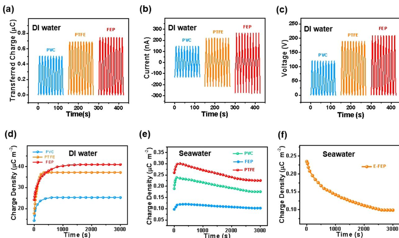
**Figure 3.** Characterization of performances of the DL-TENG. (a) Transferred charges, (b) short-circuit current, and (c) open-circuit voltage of the DL-TENG with different dielectric materials. (d) Charge density changing curve of the DL-TENG with different dielectric materials. (e) Charge density changing curve of the SL-TENG with different dielectric materials. (f) Charge density changing curve of the SL-TENG with the electret dielectric materials.
